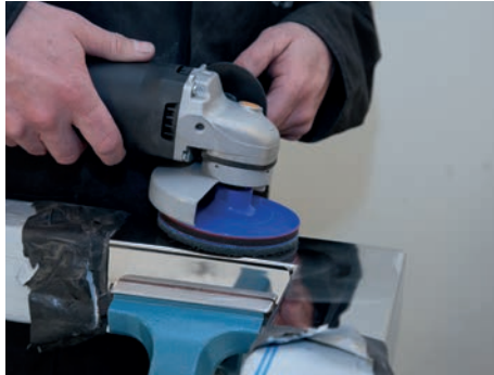
Prepolishing: ideal last step before mirror polishing.
